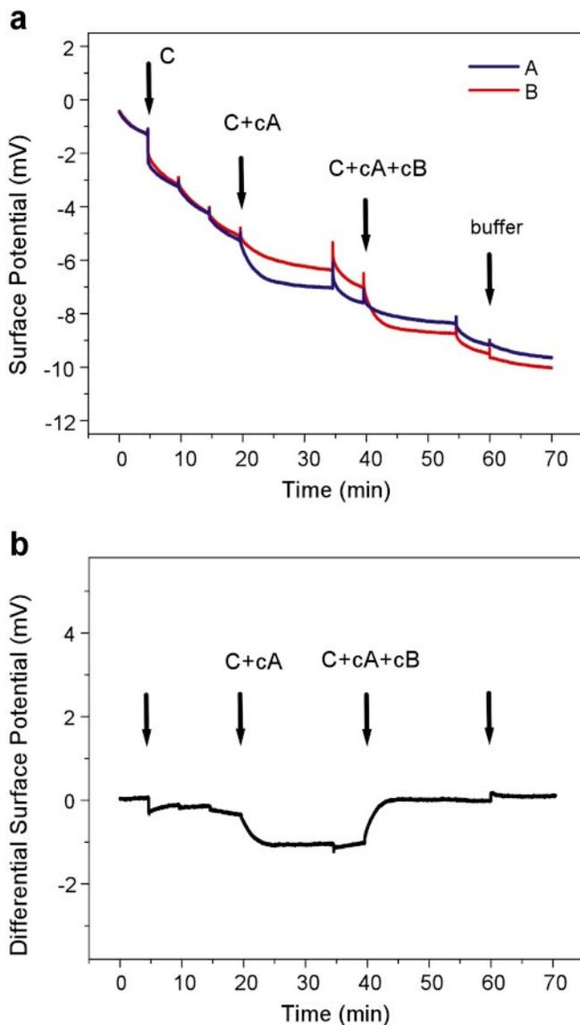
**Fig. 5.** Field-effect detection within a complex sample. Absolute surface potential (a) and differential surface potential (b) for the hybridization of 20 nM oligonucleotides *cA* to *A* and *cB* to *B* within a 10-times-higher concentration of unrelated oligonucleotides. All injections were made at a constant 200 nM concentration. Arrows indicate injections of 200 nM *C*, then 20 nM *cA* + 180 nM *C*, and then 20 nM *cB* + 20 nM *cA* + 160 nM *C*.
