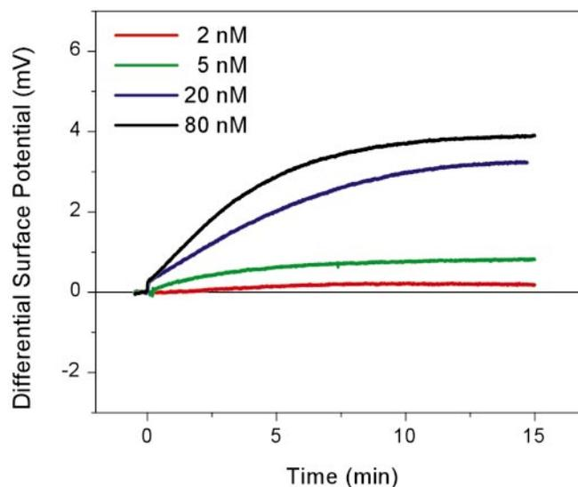
**Fig. 4.** Concentration dependence and detection limit. Shown is the differential surface potential response for the hybridization of target oligonucleotides at concentrations of 2, 5, 20, and 80 nM.
