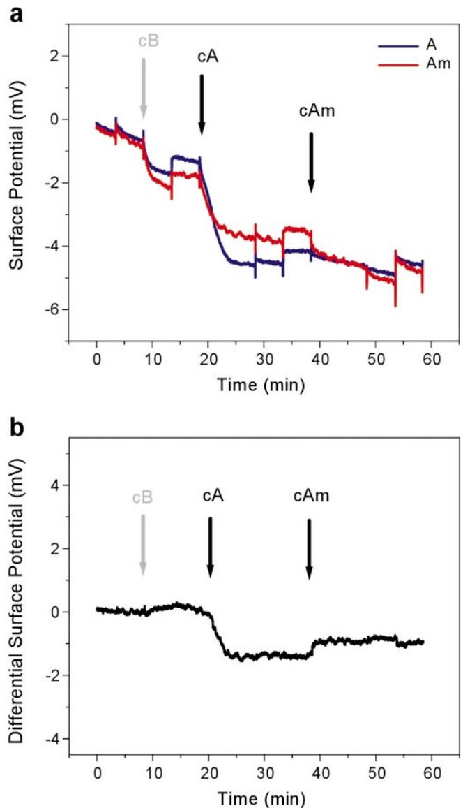
**Fig. 6.** Field-effect detection of a single base mismatch. Surface potentials from two sensors that were functionalized with probe oligonucleotides *A* and *Am*, which differ only in a single base. Control solutions with noncomplementary target oligonucleotide *cB* show no differential signal, whereas injection of 80 nM of complementary sequences *cA* and *cAm* both show a distinct hybridization signal. (a) Absolute surface potential. (b) Differential surface potential.
