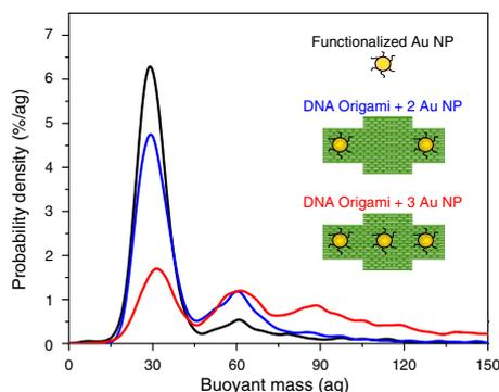
**Fig. 5.** Buoyant mass measurements of DNA origami-gold nanoparticle assemblies. Buoyant mass distributions (kernel density estimates) of functionalized 15-nm gold nanoparticles (Au NP) with ssDNA (black) mixed with DNA origami structures with two binding sites (blue) and DNA origami structures with three binding sites (red).
